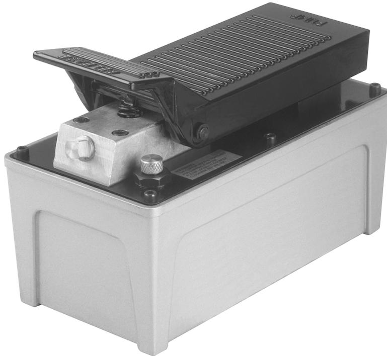
*Description: The 2510A air/hydraulic pump is designed to have a maximum capacity of 690 bar (10,000 psi). It has a 2-stage release mechanism, internal relief valve, and 1606 CC (98 cu. in.) of useable oil. It pumps, holds, or releases a load with pedal control.*
