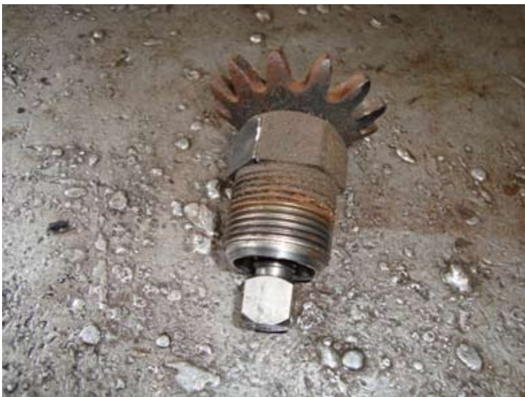
Release valve. Our particular style uses a flat recessed seat that uses a steel ball as the release valve. There are different models and yours might have a needle valve instead of this one. If that is the case, there will not be a small ball as indicated by the next picture. Remove the ball and keep it separate.
