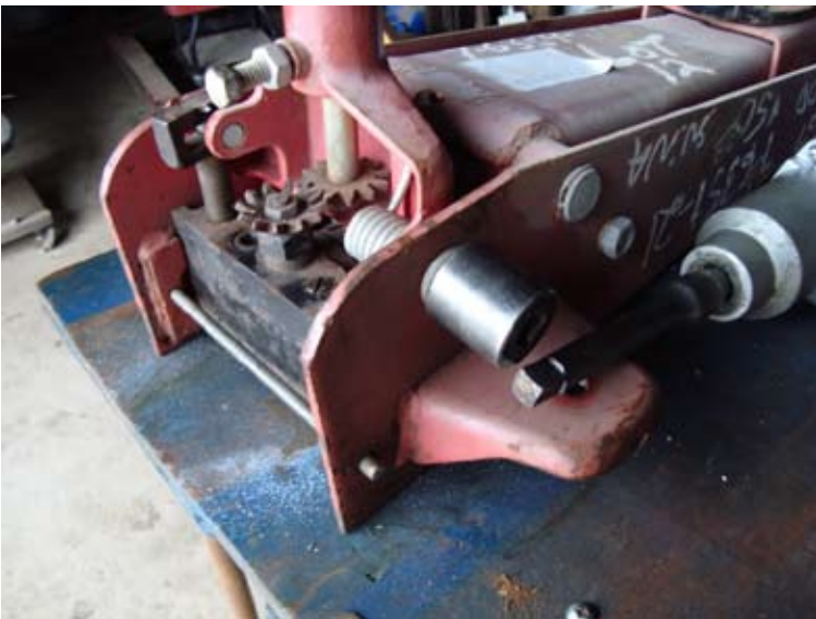
Start by removing the handle assembly. This particular jack requires a 15/16" socket to remove the handle assembly.
