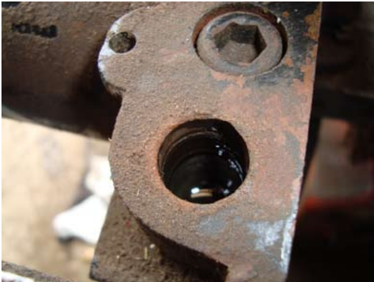
Pump hole with seals inside.
