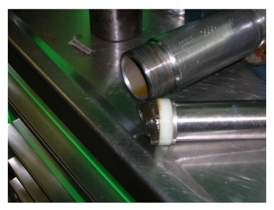
Easy to spot the problem with this one: the main seal is ripped from the center section along half of its diameter.
