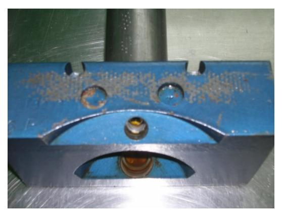
Next up are the pressure and safety valves under these expansion plugs. Center-punch the expansion plugs and remove them.
