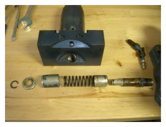
Pump assembly removed from the jack and partially disassembled as well as the release assembly/u-joint.
