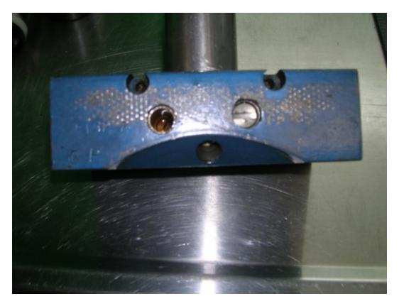
Here are the expansion plugs removed and ready to start with removing the valves. The valve on the left is the safety valve and the one on the right is the pressure/suction valve.
