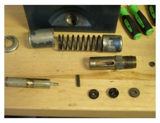
Completely torn apart pump assembly. Take your time when driving the retaining pin out and everything should go fine.
