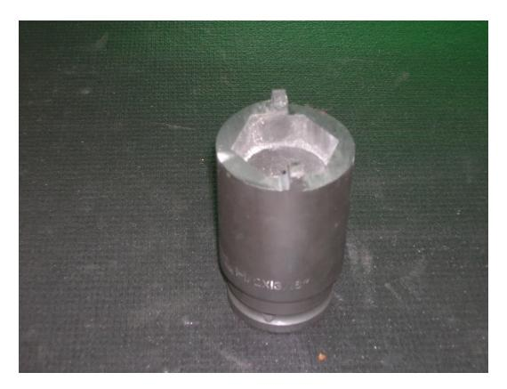
Next up was the ram but I did not have a homemade socket for this particular tank nut. I usually make one from schedule 80 or 120 pipe, a piece of plate and a nut welded to it but this time I decided to cheat. The local bargain tool store had some VERY cheap Chinese Budd sockets on sale so ... 15 minutes with a cutoff wheel, a little file work to make it fit.
