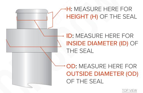
Note: For accurate measurements, please measure the metal ram, not the old seal.
