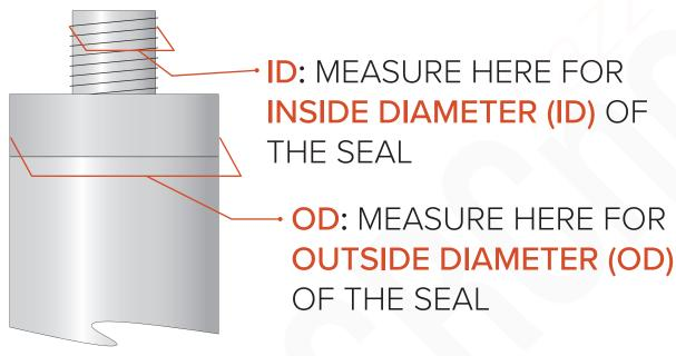
Note: For accurate measurements, please measure the metal ram, not the old seal.
