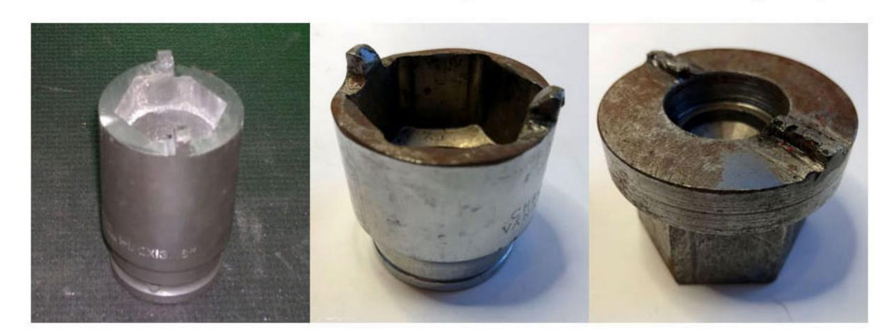
This particular tank nut needs a homemade socket for this job. You can make one from schedule 80 or 120 pipe, a piece of plate and a nut welded to or this way, with a socket. The local bargain tool store had some VERY cheap Chinese sockets on sale so ...
